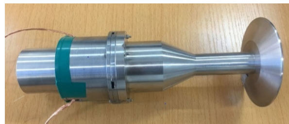
Figure 18. The prototype of the giant magnetostrictive transducer.
