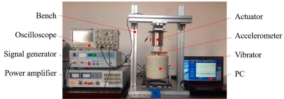
**Figure 13.** Vibration experimental setup.
