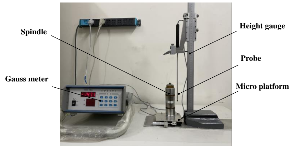
Figure 8. Test platform of magnetic induction strength.
