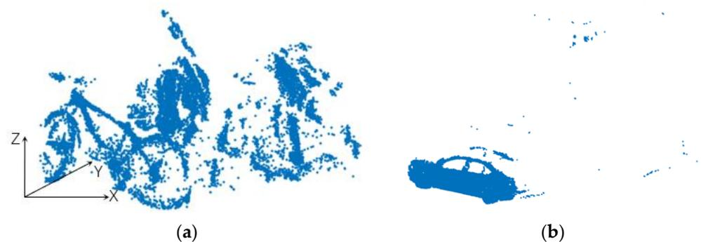
**Figure 15.** Point clouds reconstruction under the Mask-RCNN masking: (a) 3D point clouds of the 2D segmented bike; (b) 3D point clouds of the 2D segmented car.
