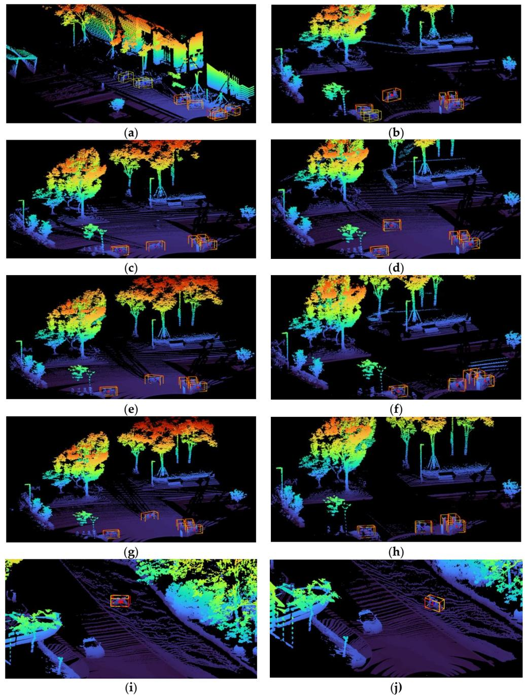
**Figure 24.** Localization results of the bikes. The yellow box is the ground truth of the bikes, and the red box is the results estimated by T-Net: (a–j) the corresponding localization results of ten scenes in Figure 21.
