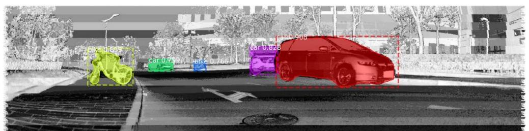
**Figure 26.** The 2D segmentation results from Mask RCNN of the outdoor scene.
