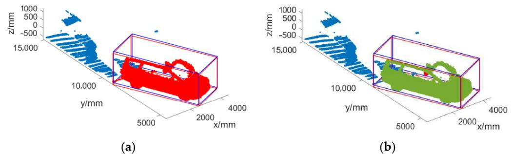
**Figure 34.** Comparison between the ANFIS method and Frustum-Pointnet [24], where the blue box is the ground truth, and the red box is the estimated results: (a) with outlier exclusion by ANFIS; (b) with the segmentation by Frustum-Pointnet.
