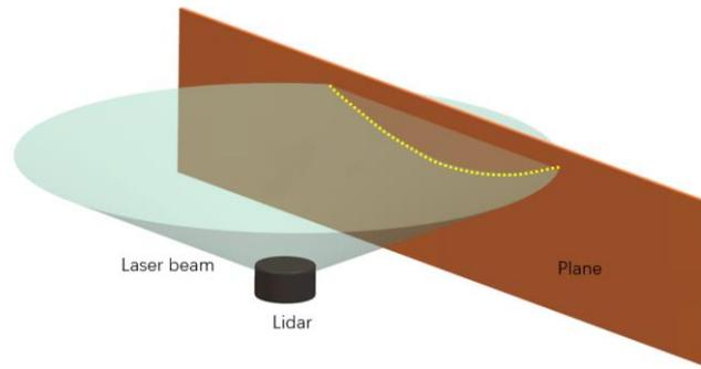
Figure 7. The measured curve on a vertical plane by a single laser beam.
