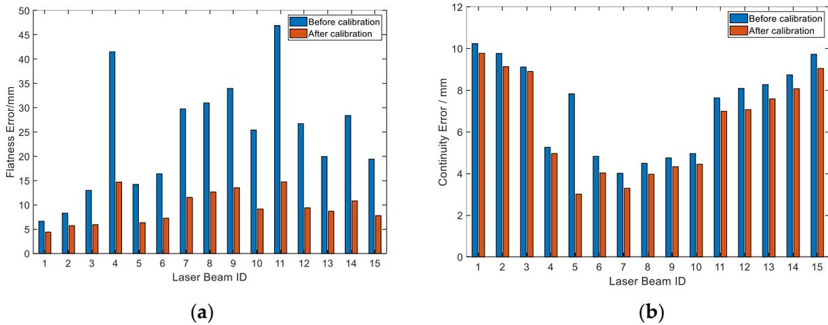
**Figure 10.** Errors changes of plane 1 before and after calibration: (a) Flatness error change of each point cloud block. (b) Continuity error change of each point cloud block.
