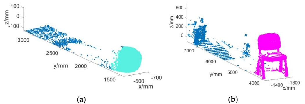
Figure 31. The ANFIS results in the indoor scene: (a) the ANFIS results of the sports ball in Figure 30 with the same mask color; (b) the ANFIS results of the chair in Figure 30 with the same mask color.
