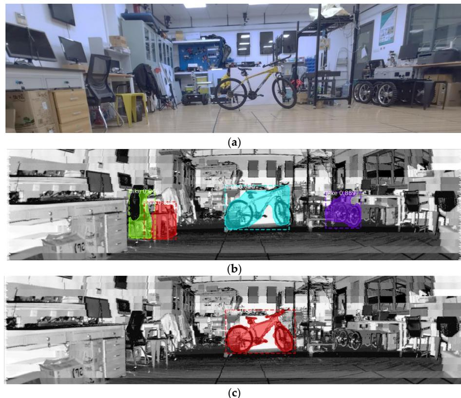
**Figure 13.** Bike segmentations using the Mask-RCNN before and after the transfer learning in the indoor scene: (a) the RGB image in the indoor scene; (b) segmentation of bike before transfer learning; (c) segmentation of bike after transfer learning.
