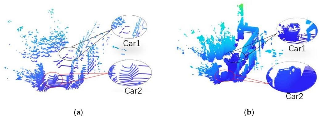
**Figure 2.** Comparison between point clouds with and without dense scanning system: (a) Original LiDAR point cloud from 16-line 3D LiDAR; (b) Point cloud with the dense scanning system.
