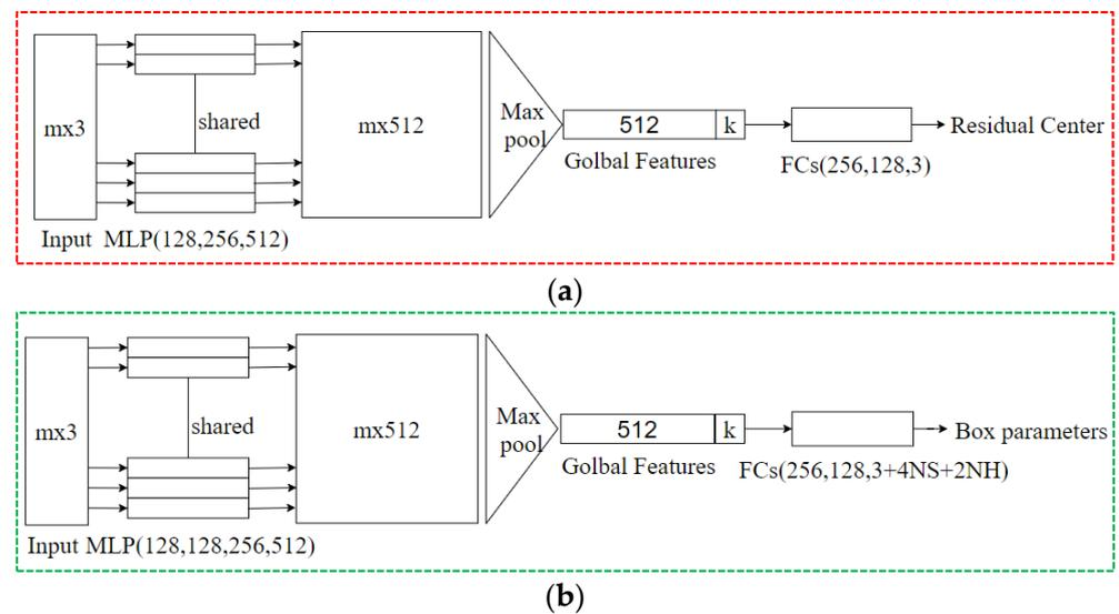
**Figure 18.** Localization Networks [24]: (a) T-net for estimating residual center; (b) Amodel 3D Box Estimation Net.
