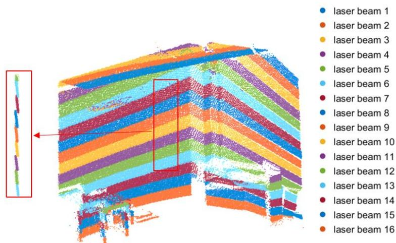
**Figure 5.** Uncalibrated dense point cloud.
