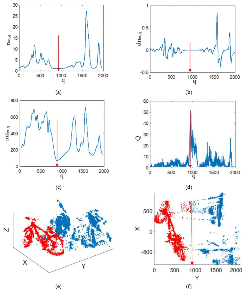
**Figure 17.** Truncating results for the 3D bike point cloud of Figure 13a: (a) the input curve of  $y_{os\_q}$ ; (b) the input curve of  $n_{os\_q}$ ; (c) the input curve of  $dn_{os\_q}$ ; (d) the output curve of  $mz_{os\_q}$ ; (e) the side view of the bike segmentation result; (f) the bird view of the bike segmentation result.
