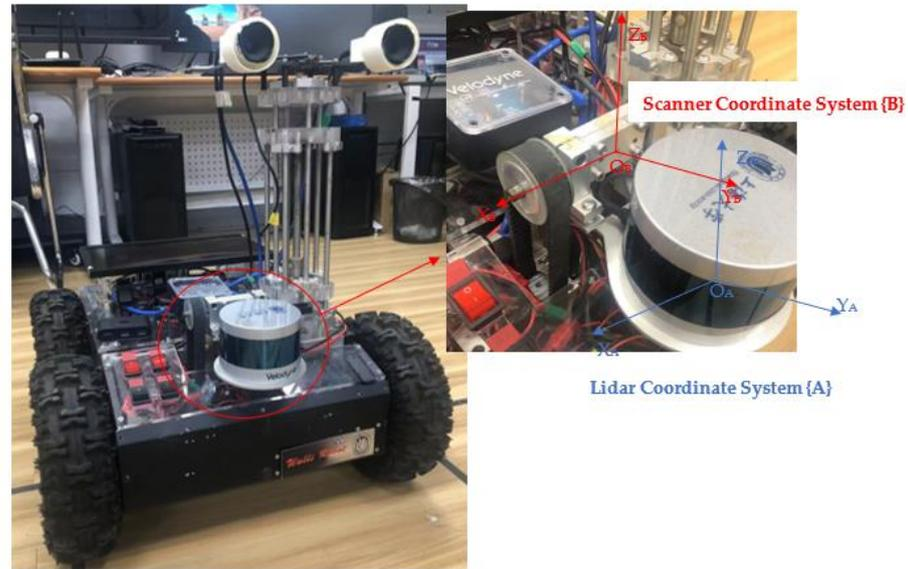
**Figure 20.** The dense scanning system installed on a mobile robot.
