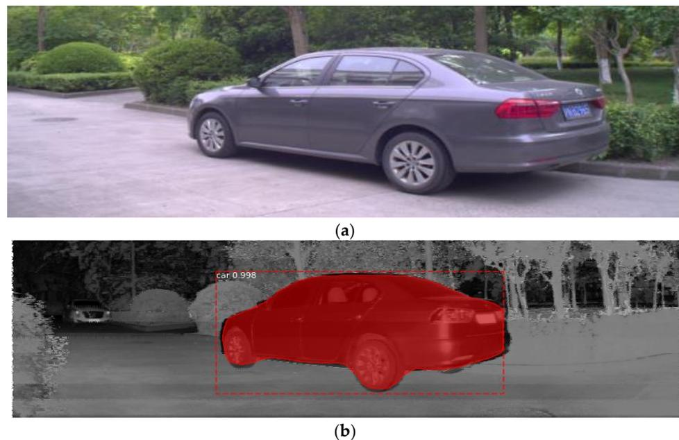
**Figure 14.** Segmentation result in outdoor experiment: (a) the RGB image in the outdoor scene; (b) segmentation for the ReV image of a car in the outdoor scene.
