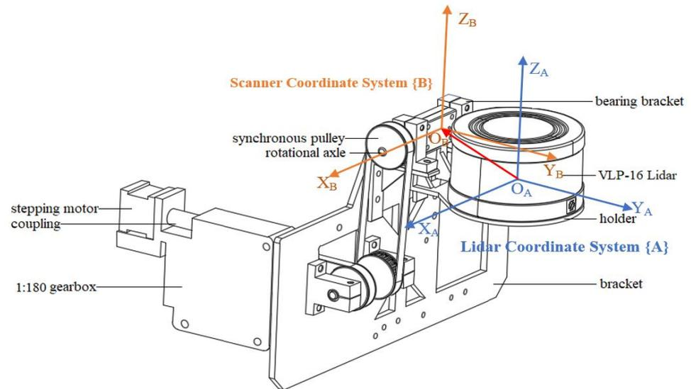
**Figure 3.** Mechanical design of the dense scan system.
