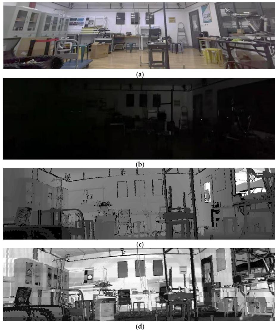
**Figure 12.** Camera and LiDAR image comparison in an indoor scene: (a) the image by a camera under normal lighting conditions; (b) the image by a camera under very weak lighting conditions; (c) the RV Image by our dense scanning system under very weak lighting conditions; (d) the ReV. Image by our dense scanning system under very weak lighting conditions.
