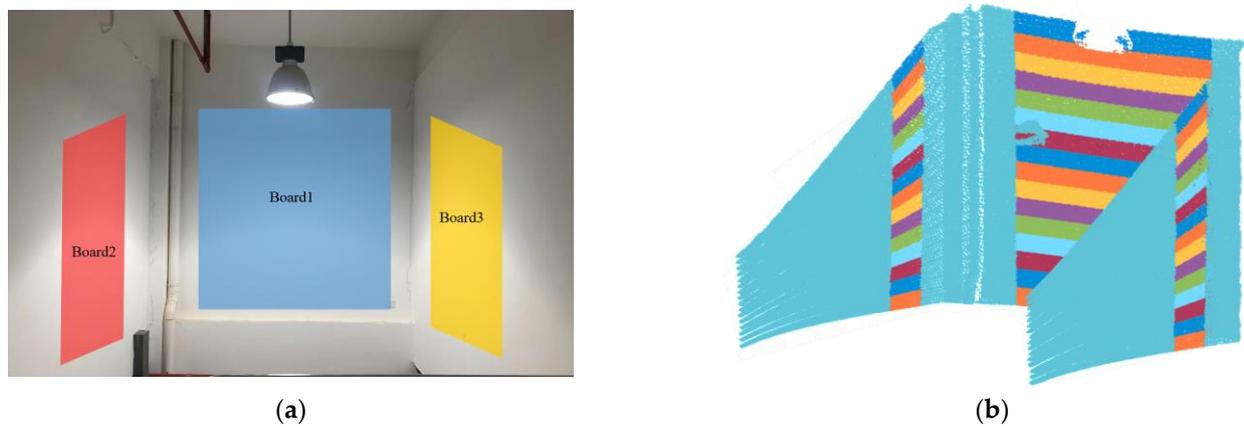
Figure 9. U-shape Experiment wall scene: (a) Experimental scene. (b) Point clouds for calibration.
