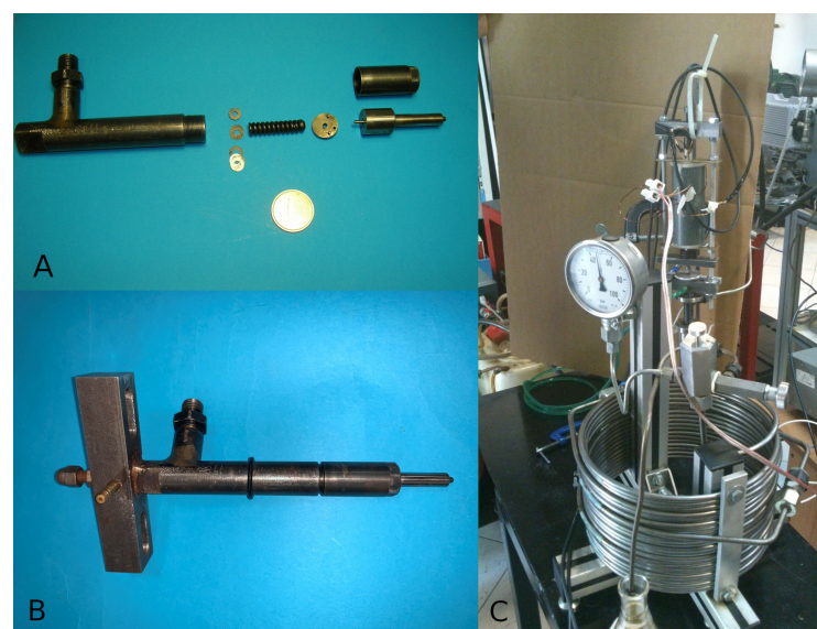
Figure 2. (A) The exploded structure of the commercial injector with a spring mechanism for the nozzle closure (1€ coin is shown as dimension reference); (B) the modified injector with iron bars and the steel rod that extends the original needle; (C) the experimental setup with the injector driven by the magnetostrictive actuator allocated on the Bosch tube for the fuel injection rate measurements.
