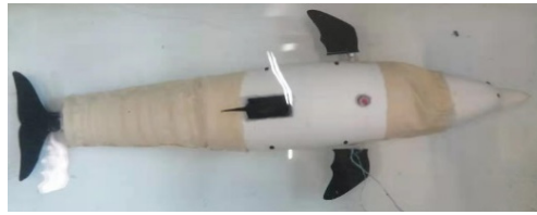
Figure 22. Experimental diagram of water tightness of dolphins.
