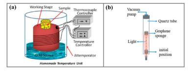
**Figure 7.** (**a**) Schematic of the preparation of bulk graphene sponge by hydrothermal method [77]. Permission from Springer Nature. (**b**) The schematic diagram of the vertical rise of graphene sponge under laser irradiation.
