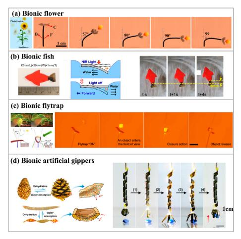
**Figure 9.** Nature-inspired light-powered soft robot. (a) Bionic flower prepared by flexible actuator [93]. Permission from RSC Publishing. (b) Fishtail-inspired robotic fish actuator design [83]. Permission from American Chemical Society. (c) Grasping robot inspired by flytrap [92]. Permission from Springer Nature. (d) Design and lifting process of the mechanical arm [47]. Permission from American Chemical Society.
