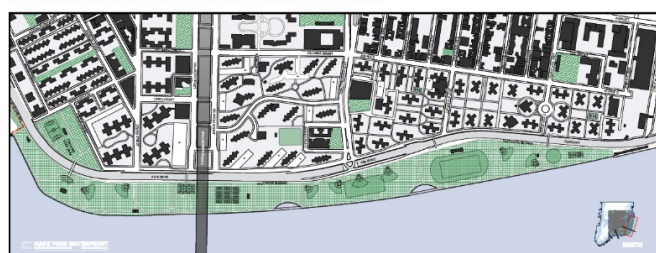
Figure 3. The BIG “U” aimed at creating large-scale protective infrastructure while ensuring meaningful community engagement. (a) Plan of New York with projected flooded areas by 2050; (b) Section of the Bridging Berm raised 14 feet along the FDR Drive. Source: (BIG 2013).
