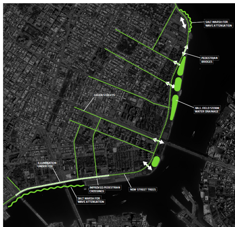
Figure 2. The East River Blueway Plan included natural beaches and other recreational amenities along the shoreline and wetlands to mitigate stormwater runoff. Source: (BIG 2013).
