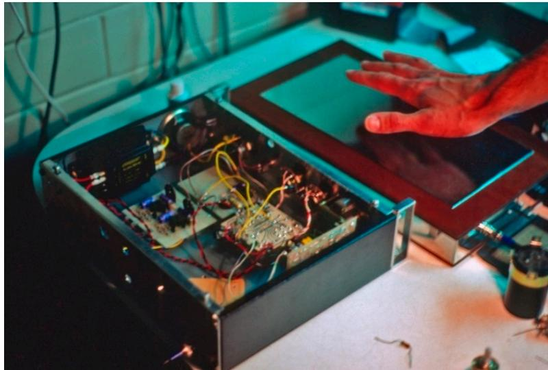
**Figure 12.** Internal view of Ostoja’s theremin showing electronics. Published with permission. Image courtesy Russell Dahms.
