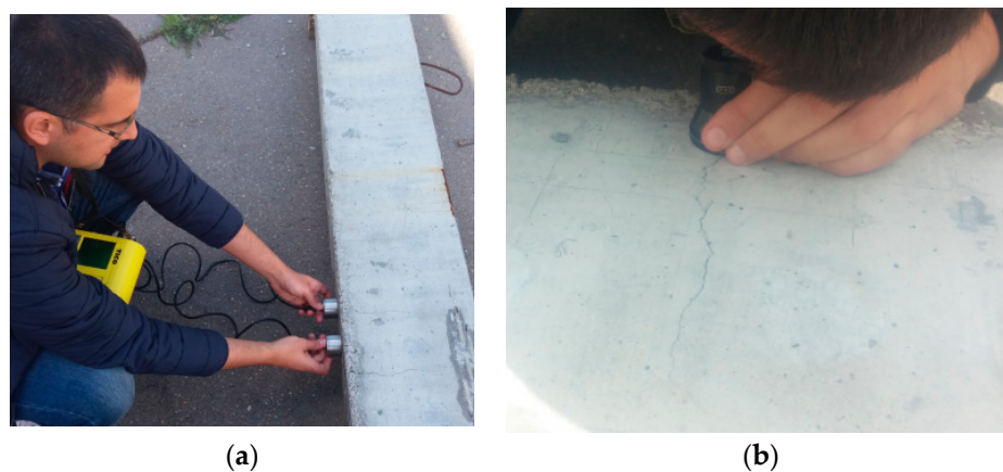
Figure 5. Determination of crack depths in reinforced concrete elements by ultrasonic testing instrument Proceq-TICO (a), visually by using crack magnifier Proceq (b) (personal archive).
