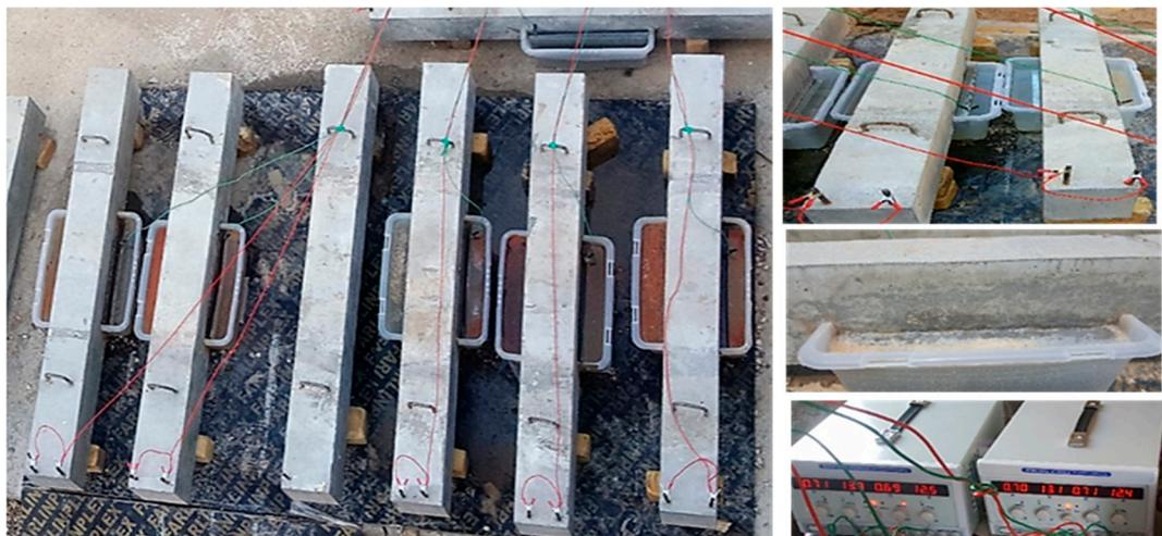
Figure 2. Acceleration corrosion process.
