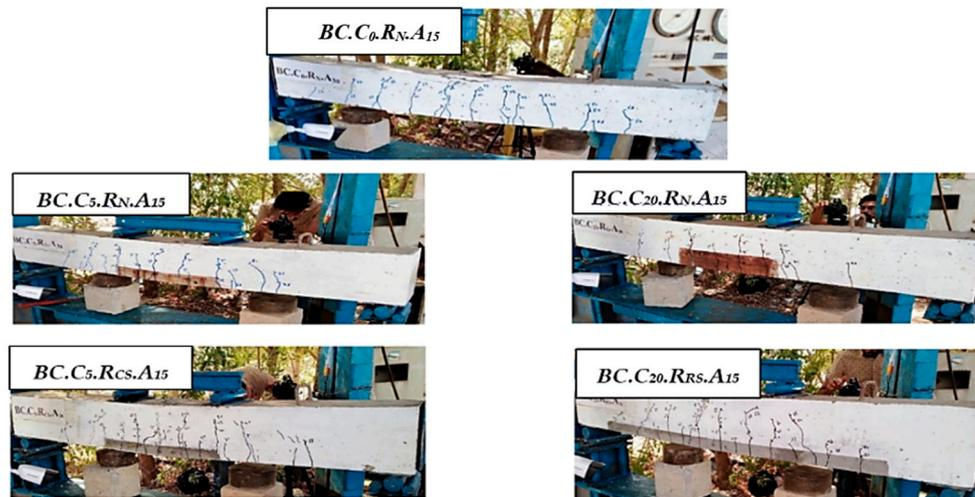
Figure 7. Cracking patterns at failure for specimens in Group B.
