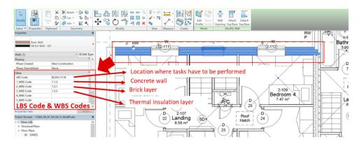
Figure 5. LBS and WBS codes displayed in the proprieties of a wall object.
