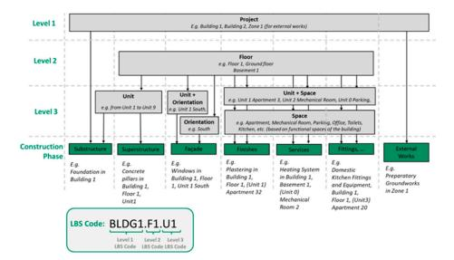
Figure 3. Location breakdown structure of the construction project's location hierarchy.
