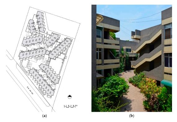
**Figure 3.** (a) Site Plan of Yamuna Apartments with housing blocks placed along four radially-converging streets [19]; (b) housing units overlooking the narrow pedestrian streets in Yamuna Apartments (Photo: Author).
