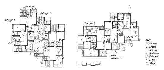
Figure 4. Floor plans of the three unit types with arrows depicting cross-ventilation [19].
