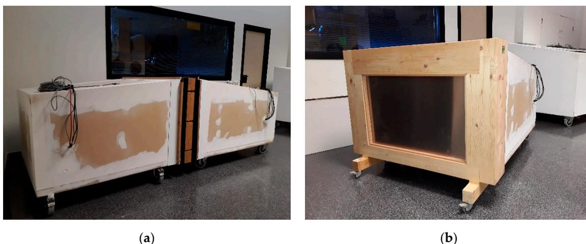
**Figure 1.** Completed reduced sized transmission chamber: (a) the two rooms with the sample holder in between; (b) view of the sample holder.
