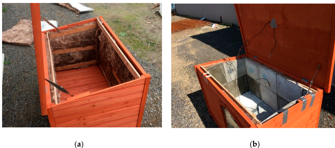
Figure 2. Test hut set up: (a) installation of insulation to the interior walls; (b) PCMCB installed on the interior surfaces.
