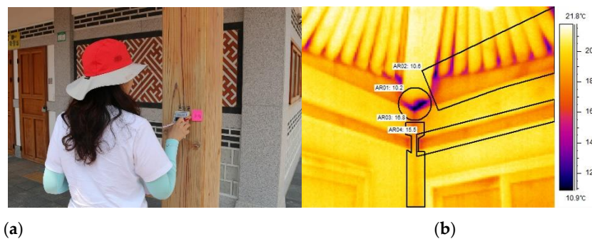
Figure 3. Monitoring method for the Hanok maintenance: tool inspection by automated devices. (a) Measurement using devices; (b) Analysis with infrared photography.
