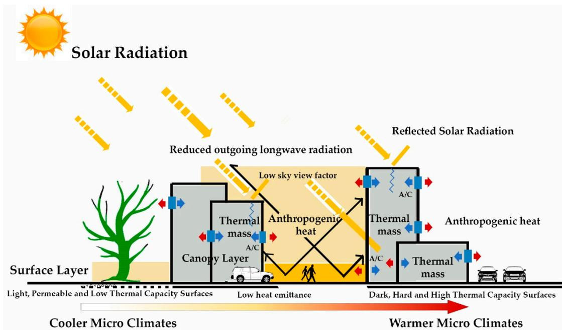
**Figure 3.** Urban Canopy Layer influenced by the building density and surface coverage. Source: A. Soltani and E. Sharifi, 2017.
