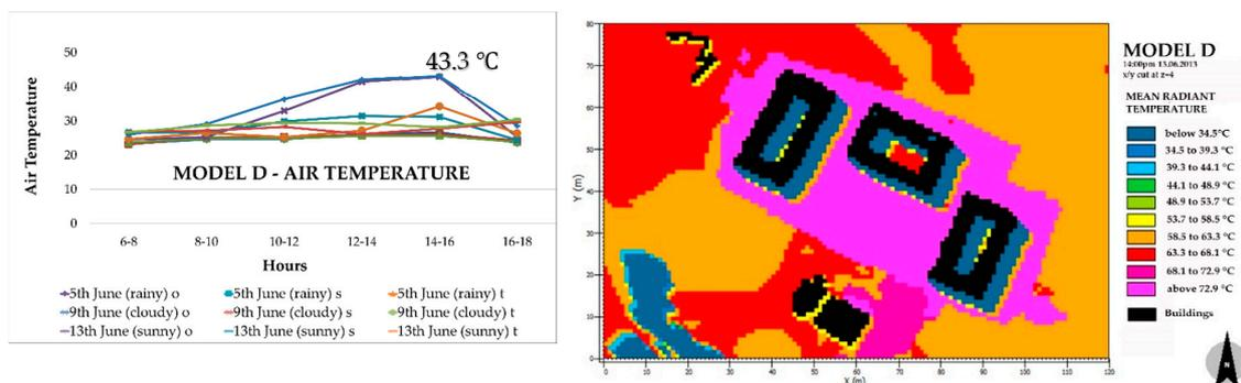
Figure 4. Model D—Square Plot Microclimate.
