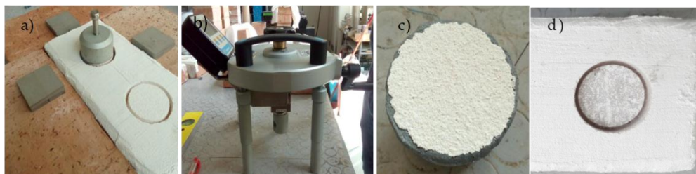
Figure 3. (a) Sample with steel cylinders connected to the instrument for the measurement of adhesion strength; (b) tear-off-adhesive tester; (c) steel cylinders after test; (d) sample after test.
