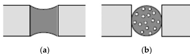
**Figure 8.** Conventional solution components: (a) Sealing compound (caulking); (b) Porous gasket (foam backing rod) [32].
