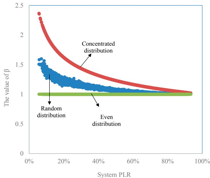
**Figure 3.** The value of  $\beta$  (coupling effect) under three types of load distribution conditions.
