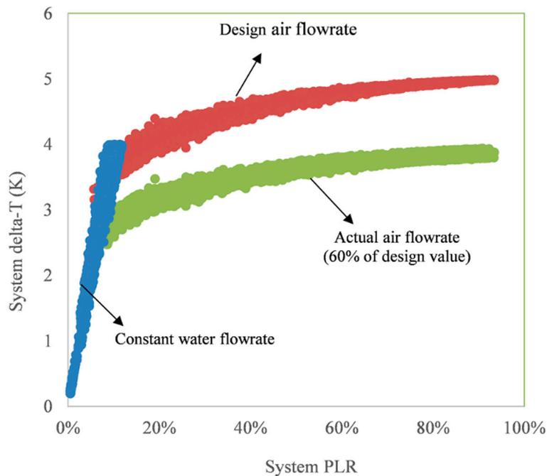
Figure 4. Performance map of system delta-T under typical faults.
