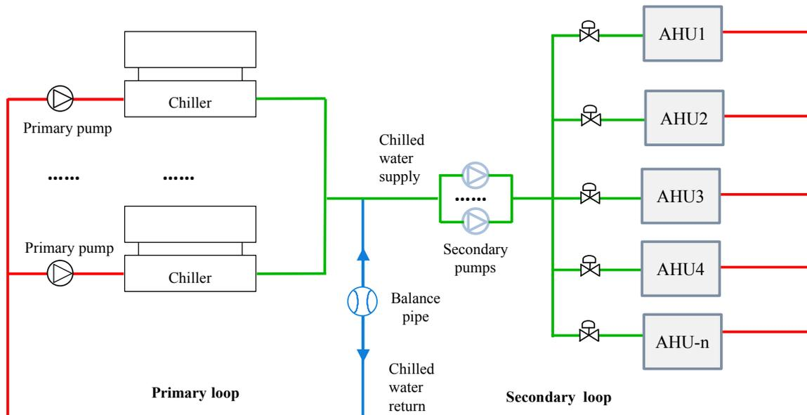
**Figure 1.** Schematic of a typical primary-secondary chilled water system.
