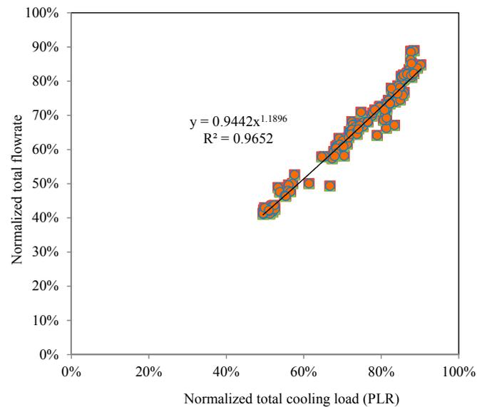
**Figure 5.** Parameter identification of AHU using operational data of three days.
