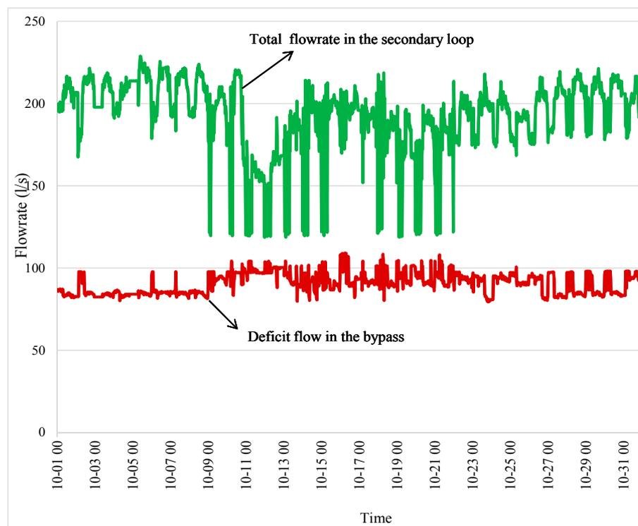
Figure 8. Actual flowrate in the secondary loop and in the bypass pipe.
