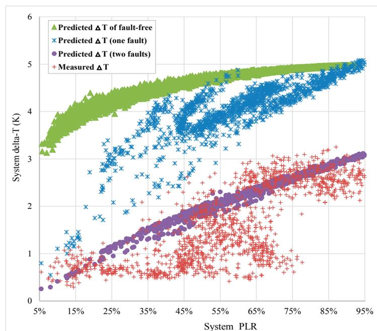
**Figure 6.** Predicted and measured system delta-T under part load conditions.
