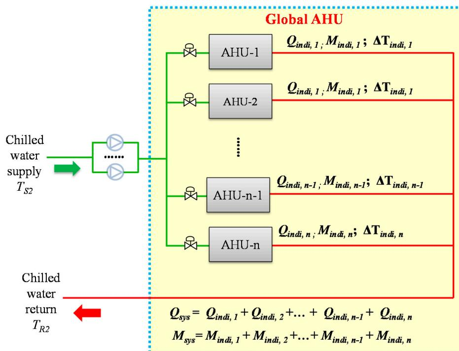
Figure 2. Scheme for development of global air handling unit (AHU) model.
