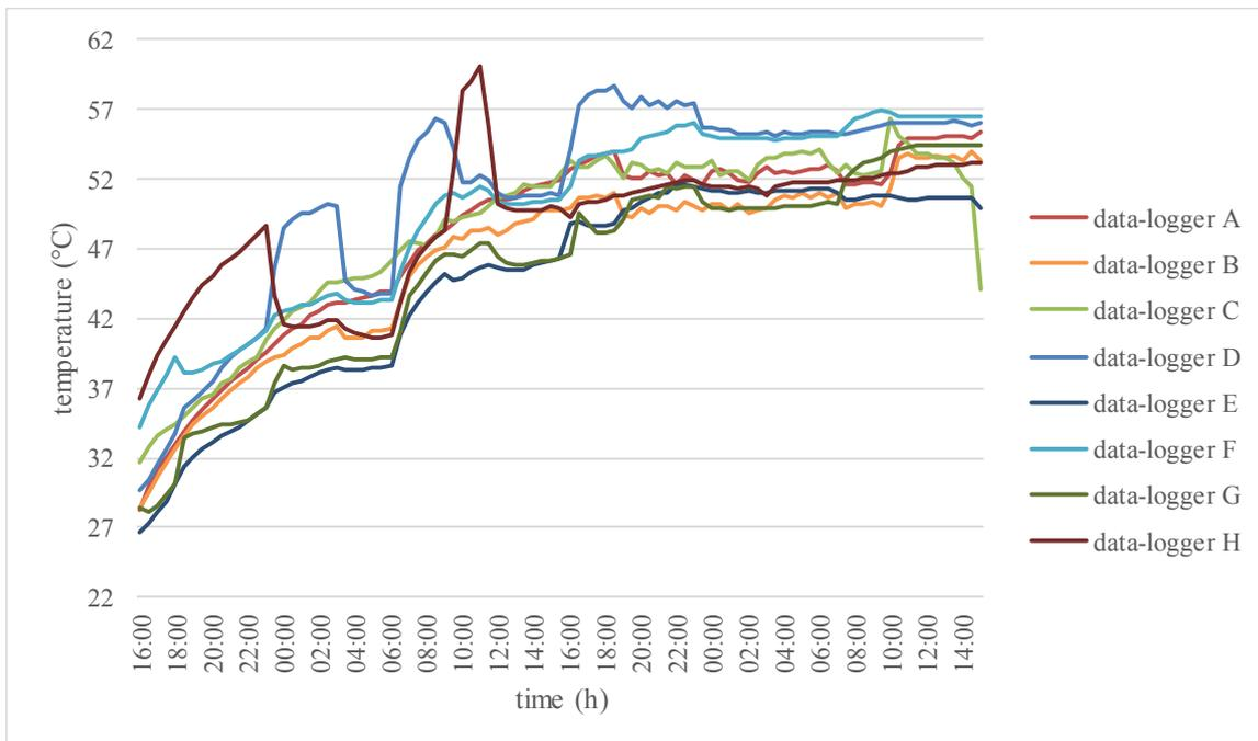
**Figure 6.** Indoor air temperature detected by the temperature probes during heat treatment (24/04/2014–26/04/2014).
