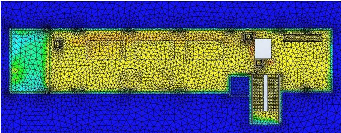
Figure 4. Automatic mesh sizing.
