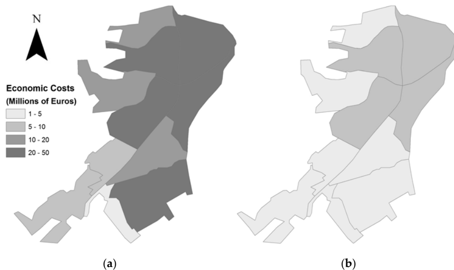
Figure 13. Distribution of economic cost according to (a) the deterministic scenario and (b) the probabilistic scenario.
