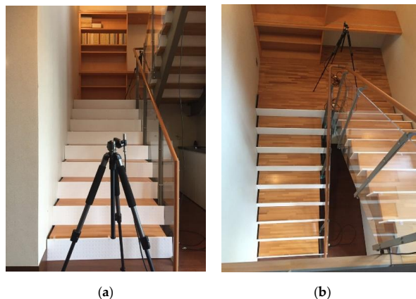
Figure 5. Sound absorption panel installation status in the riser. (a) Setup as seen from the first floor. (b) Setup as seen from the second floor.
