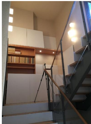
Figure 6. Sound absorption panel installation setup in the wall of landing.
