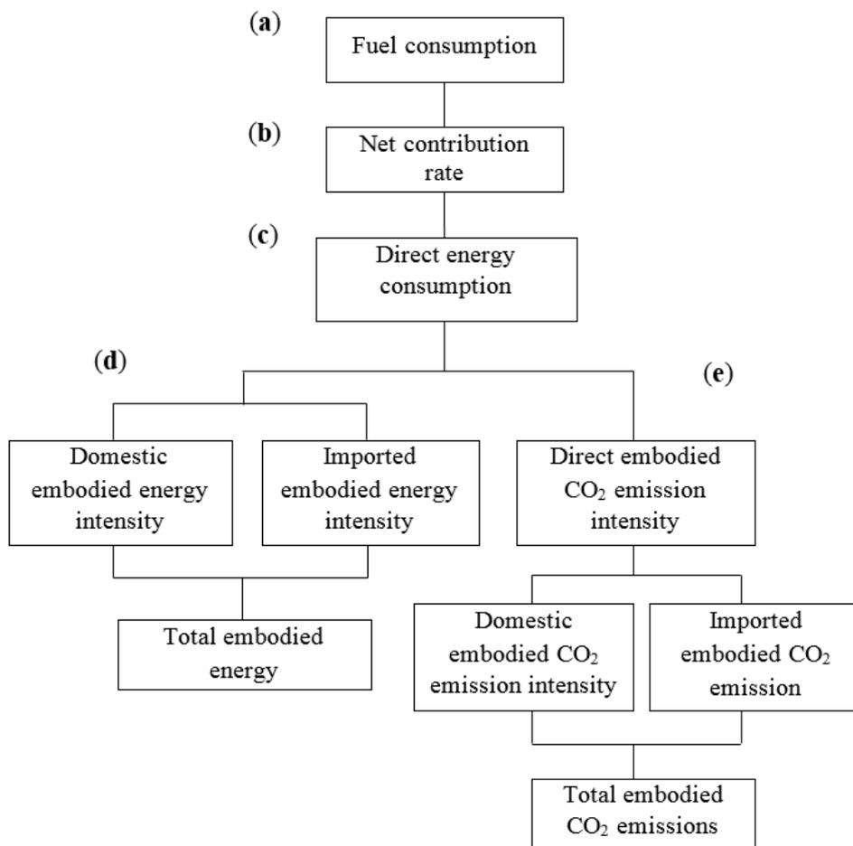
**Figure 3.** Flow chart of I-O analysis-based method for embodied energy. (a) Fuel consumption calculation, (b) determination of net contribution rate, (c) net calorific value, (d) embodied energy calculation and (e) embodied CO<sub>2</sub> emission calculation.
