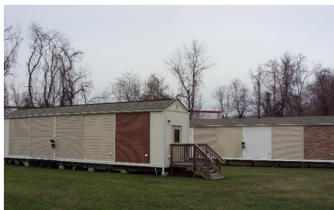
Figure 1. Test structures showing south-facing wall assemblies.
