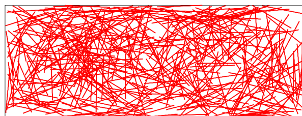
Figure 3. Random distribution of fibers for the simple tension test.
