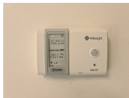
Figure 7. LoRa Mulesight AM107 sensor [11].
