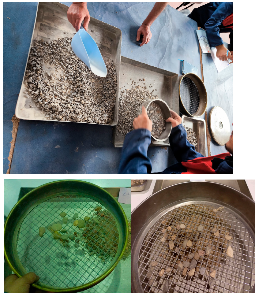
Figure 2. The aggregate materials used in the study and the corresponding sieve analysis procedures.
