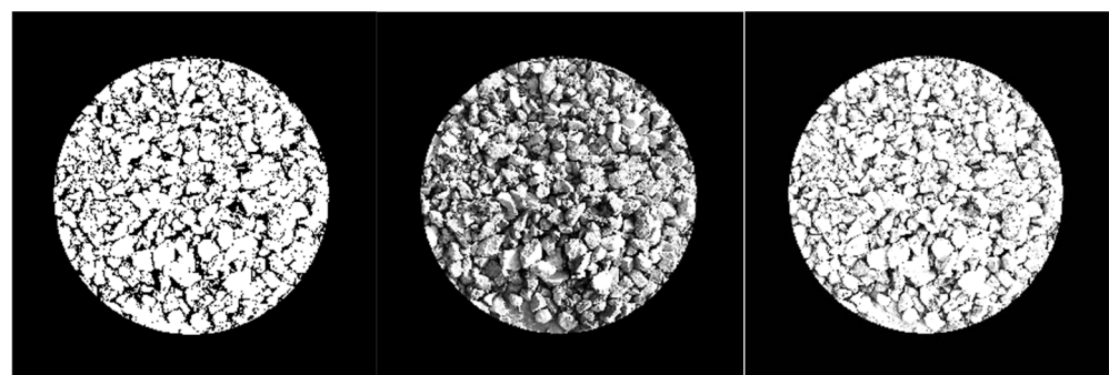
Figure 5. Grayscale preprocessed images under equal boundary conditions, selected area, histogram equation and OTSU, respectively.
