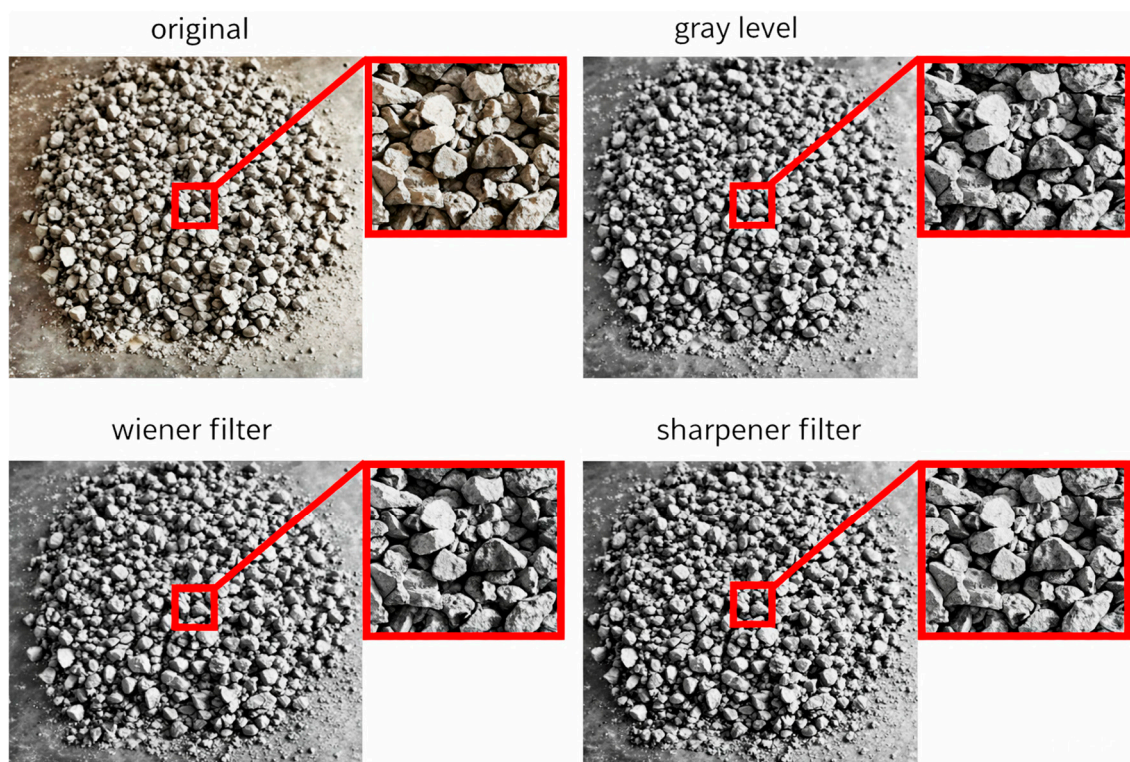
Figure 4. The vertically captured original image and its converted versions in grayscale, Wiener-filtered, and sharpener filter formats.
