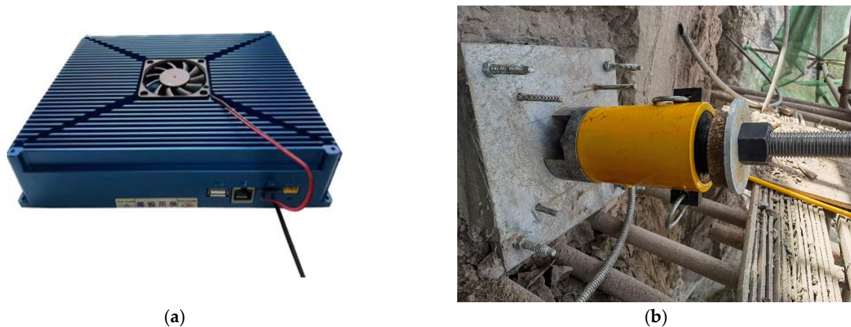
Figure 7. Tensioning and monitoring equipment. (a) Decimeter-grade ultra-weak FBG wavelength-demodulation module. (b) Tensioning apparatus.
