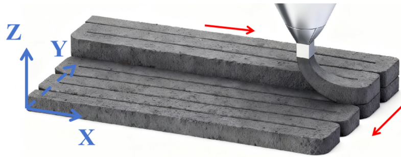
Figure 4. Schematic diagram of the direction of mechanical property testing of 3D printed specimens.
