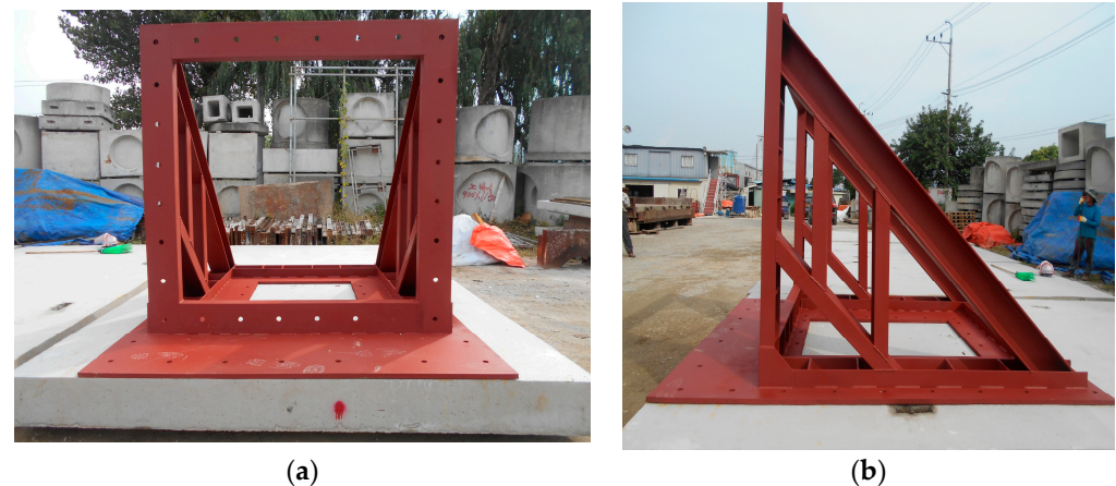
Figure 3. Fixing frame for blast experiments: (a) front view; (b) side view.
