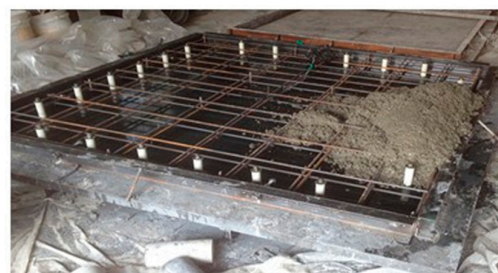
Figure 1. Reinforcement details of slab specimens: (a) reinforcement layout and spacing; (b) completed reinforcement arrangement.
