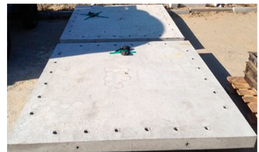
Figure 2. Fabrication process of slab specimens: (a) installation of bolt holes; (b) finished slab specimen after production.
