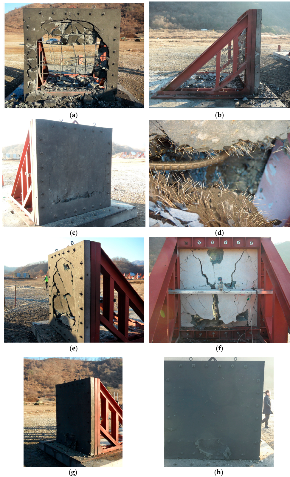
Figure 12. Experimental damage specimens: (a) NC specimen front view; (b) NC specimen side view; (c) UHPFRC front view; (d) fiber pull-out after blast; (e) O-HPC front view; (f) O-HPC back view; (g) F-SIFCON side view; (h) F-SIFCON front view.
