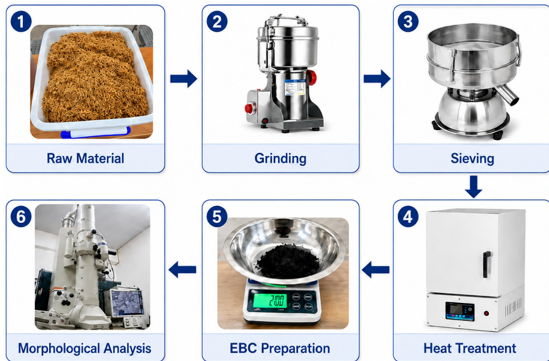
Figure 1. The process and inspection procedures for processing raw EFB into EFB biochar.
