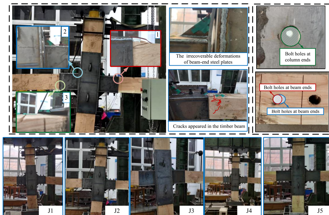
Figure 8. Specific failure patterns of specimens.
