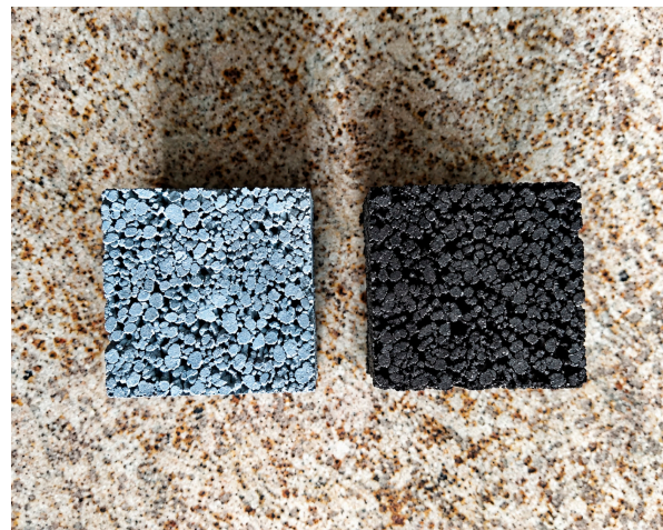
Figure 4. Photocatalytic porous concrete (left) and ordinary concrete (right).
