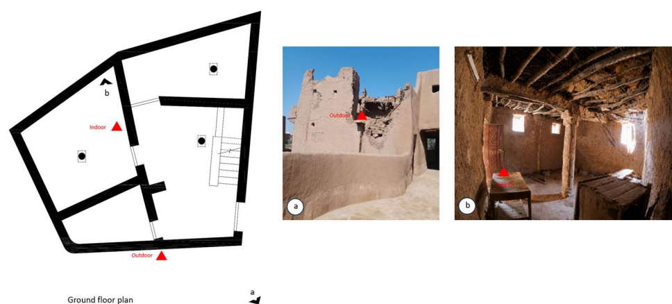
Figure 2. Ground-floor monitoring layout and field photographs of the sensor locations. (a) External sensor location; (b) Internal sensor location.
