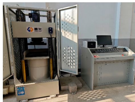
(a) Hydraulic pressure testing machine
