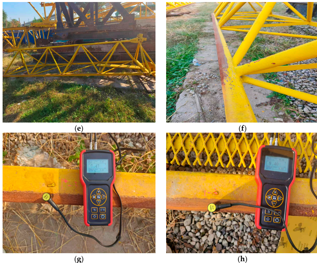
Figure 6. Field photographs of the jib with different jib segments. (a,b) The overall view and wear details of the b01 segment; (c,d) the overall view and wear details of the b03 segment; (e,f) the overall view and wear details of the b06 segment; (g,h) the measurement process.
