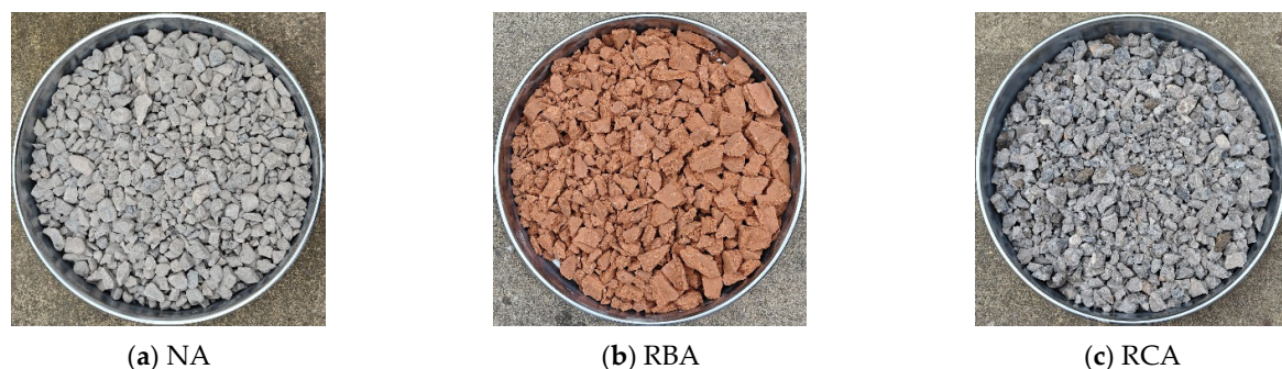
Figure 1. Surface characteristics of coarse aggregate.
