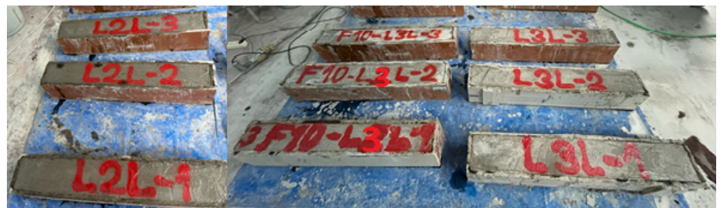
Figure 2. The fabricated low-strength RC beams incorporating various longitudinal reinforcement configurations.
