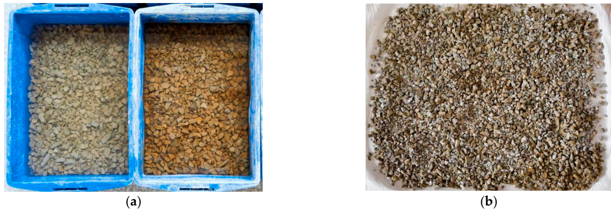
Figure 2. The process of reinforcing with flawed excavated-mass aggregates: (a) soaking process; (b) air dry process.
