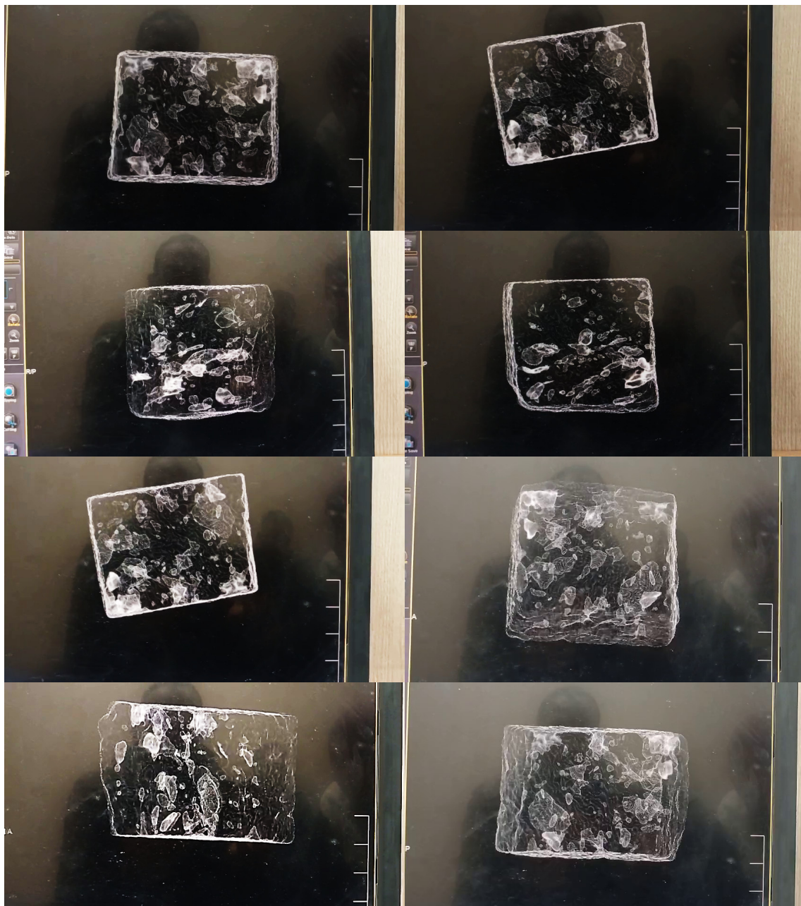
Figure 7. Representative CT sections of GO-ESTEL-treated adobe showing internal attenuation variations and visible void-related features. The images provide qualitative structural information for the treated material only; no untreated CT comparison is presented.
