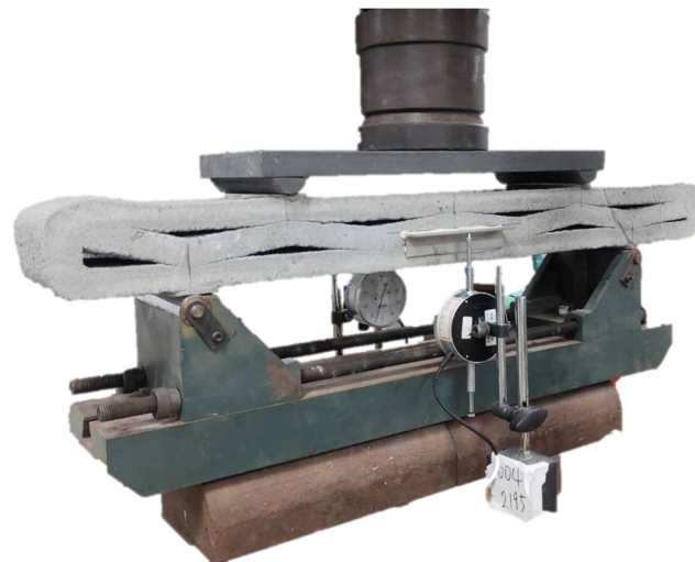
Figure 8. Experimental setup for the four-point bending test of the 3D-printed truss member.
