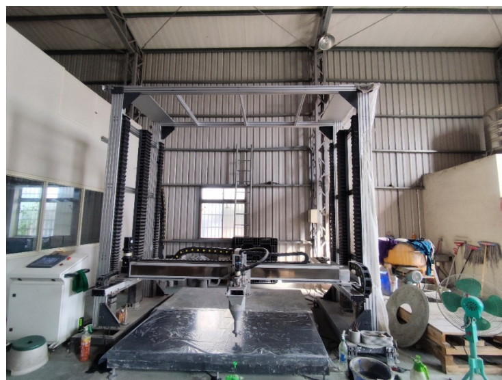
Figure 7. Gantry-type 3D printing system.
