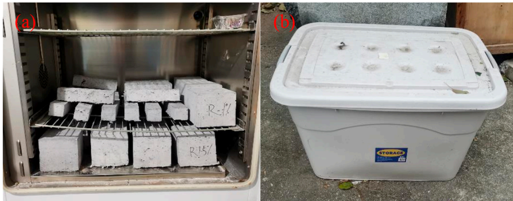
Figure 3. Sample processing: (a) Drying treatment; (b) Saturation treatment.
