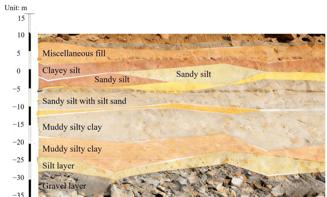
Figure 3. Engineering geological profile.
