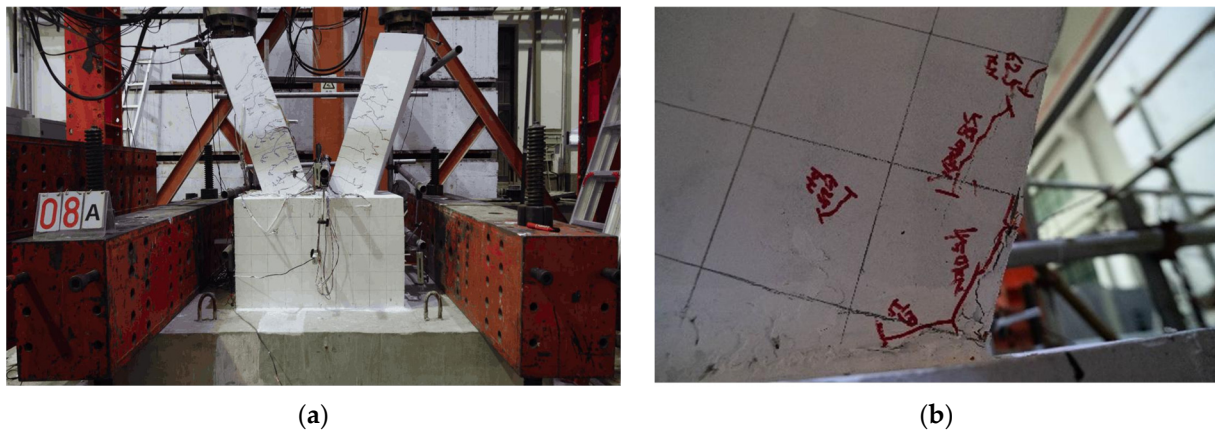
Figure 7. Failure morphology diagram of specimen JD-1 in phase 4. (a) Phase 4 integral structure. (b) Phase 4 partial view.
