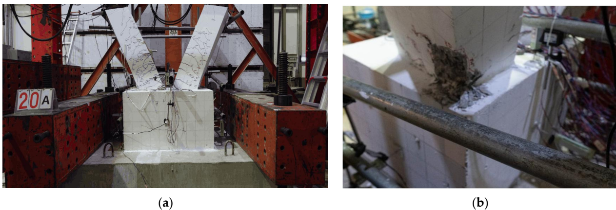
Figure 8. Failure morphology diagram of specimen JD-1 in phase 6. (a) Phase 6 integral structure. (b) Phase 6 partial view.
