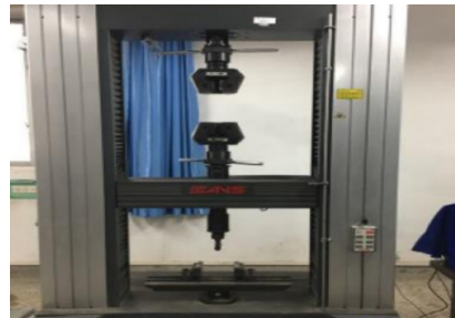
Figure 5. Flexural strength testing apparatus.
