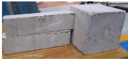
Figure 3. ECC-FLS with a foam content of 513 L/m 3 .
