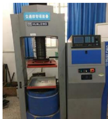
Figure 6. Compressive strength testing apparatus.
