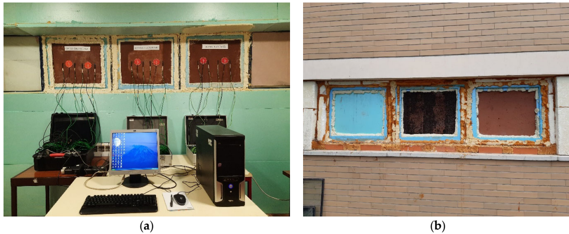
Figure 8. Thermal experimental set-up of the half-sandwich panels, AAC + extruded polystyrene ( AP_{XPS} ), AAC + insulation corkboard ( AP_{ICB} ), and uninsulated panel (ACP): (a) sealed interior view; (b) sealed exterior view.
