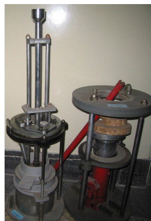
Figure 7. Soil pusher and compaction apparatus.
