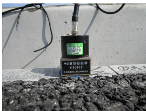
Figure 6. Photo of accelerometer (Type 941B accelerometer).
