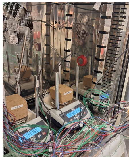
Figure 3. Cob samples inside the climatic chamber.
