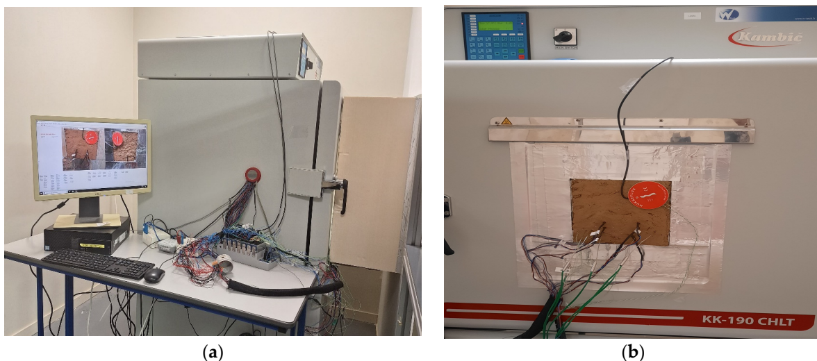
Figure 4. Experimental setup for controlled heat and humidity transfer through materials: (a) acquisition system, (b) the test bench.
